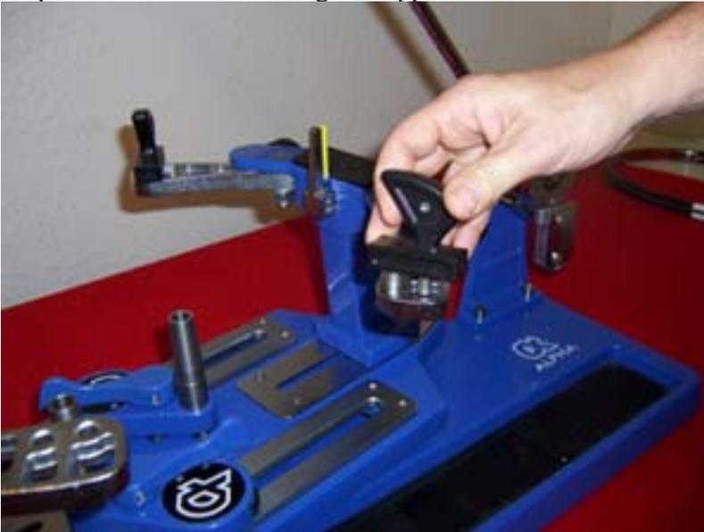
Step 4: Insert the DDS string clamp into the hosel of the clamp base, do this for both clamps.
