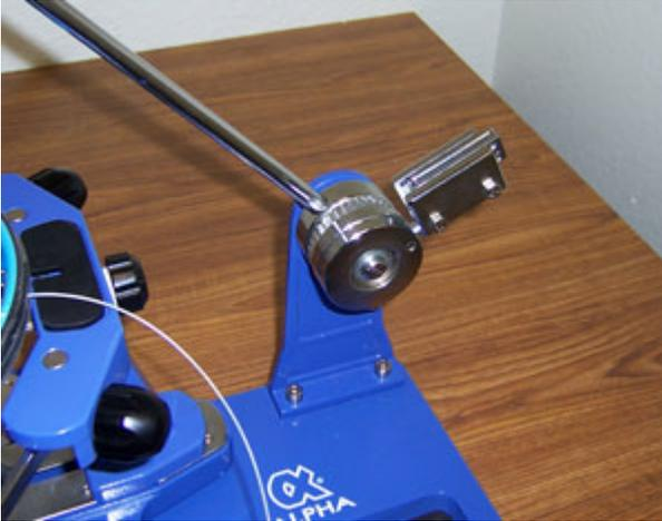
Step 5: Bring the tension bar down slowly, as the tension bar lowers, it will pull tension on the string. If the tension bar falls below the horizontal (3 o'clock) position, then raise the tension bar and lower again. When raising the bar hold the gripper still and then gently lower. Do so until the bar is in an horizontal position and the hash marks on top of the gripper match.
