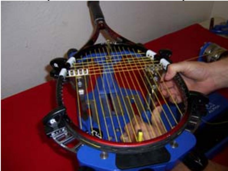
Step 14: When you complete the crosses, tie off at the appropriate tie off hole using the double half hitch.
