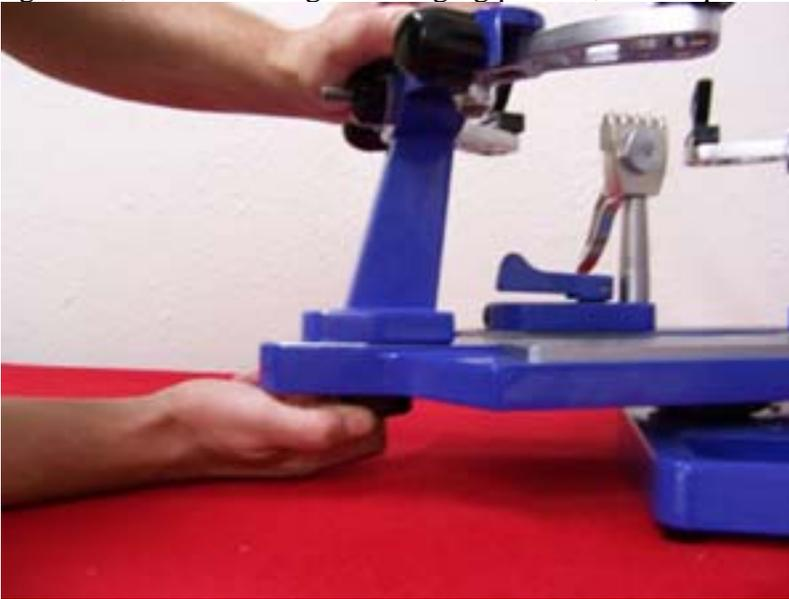
Step 2: Make sure the head (12 o'clock) and throat (6 o'clock) frame posts are positioned in between the two center-most grommets, and then adjust the black knobs until the posts are appropriately holding the frame. Make sure all 6 points are contacting the frame. Careful not to overtighten.
