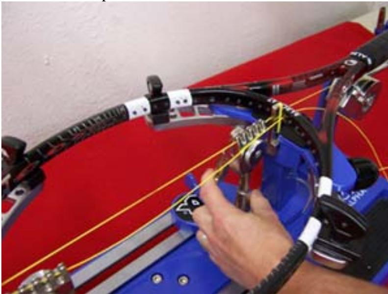
Step 7: Pull each string individually and make sure to alternate the pulling of each main. Example: Pull left main, pull right main, pull left main, etc. DO NOT pull all the mains on one side of the frame because this can cause structural damage.
