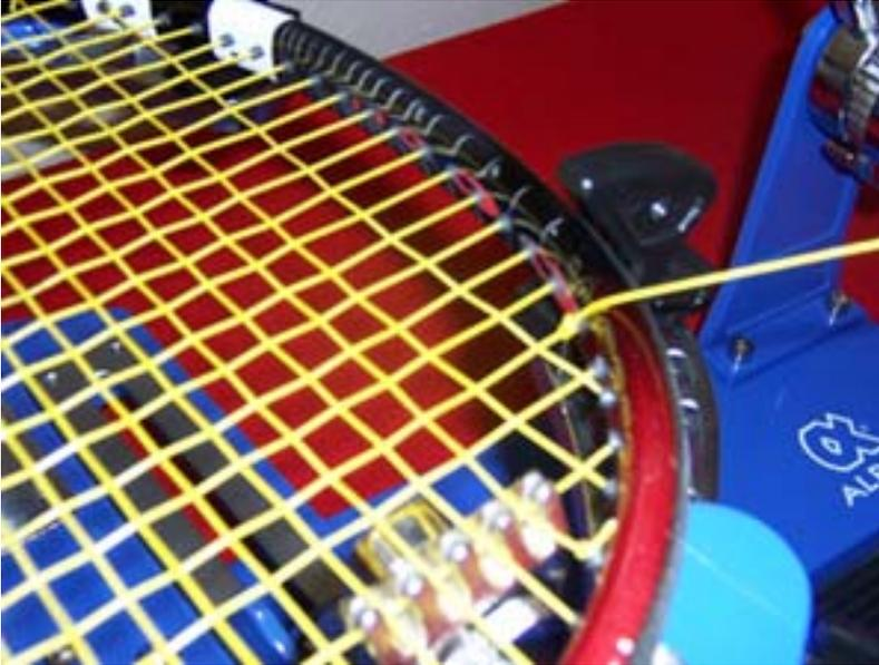
Step 15: To remove the racquet, loosen each mounting arm adjustment knob and remove the racquet.
