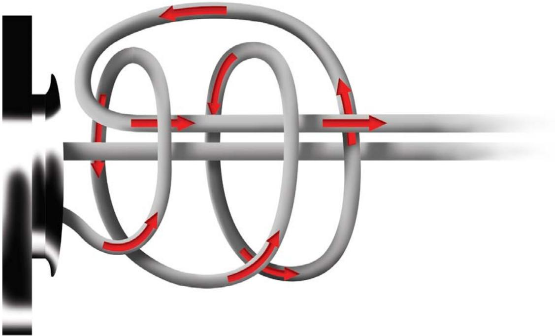
Step 13: Continue stringing the crosses making sure that you run the crosses up and down across the mains as shown in Step 11. This will eliminate premature notching of the mains. Clamp each cross as close to the frame as possible.
