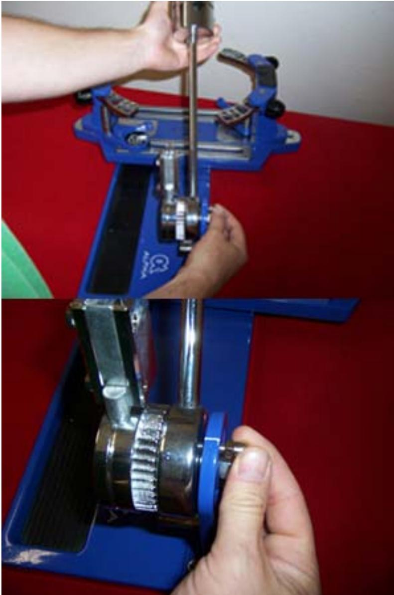
Step 2: Loosen the 12 and 6 o'clock adaptors and flip into upright position. Retighten the black knobs.
