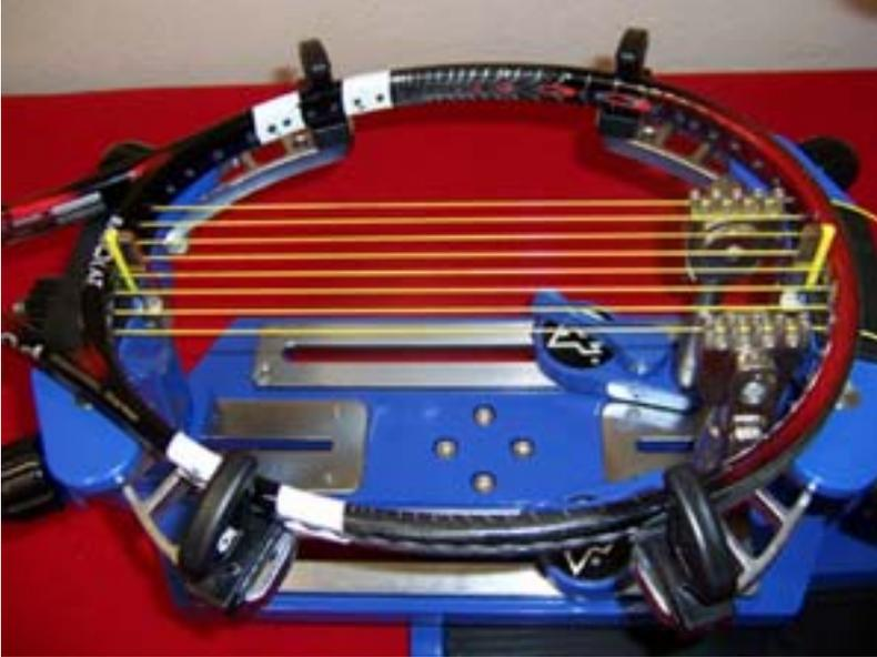
Step 8: When done pulling the mains prepare to tie off if using a two piece, or tie off the short side.
