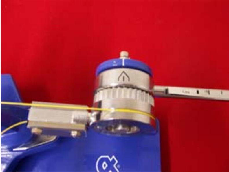
Step 6: Once tension has been achieved. Make the proper clamping adjustment. Be sure to lock the clamp base.
