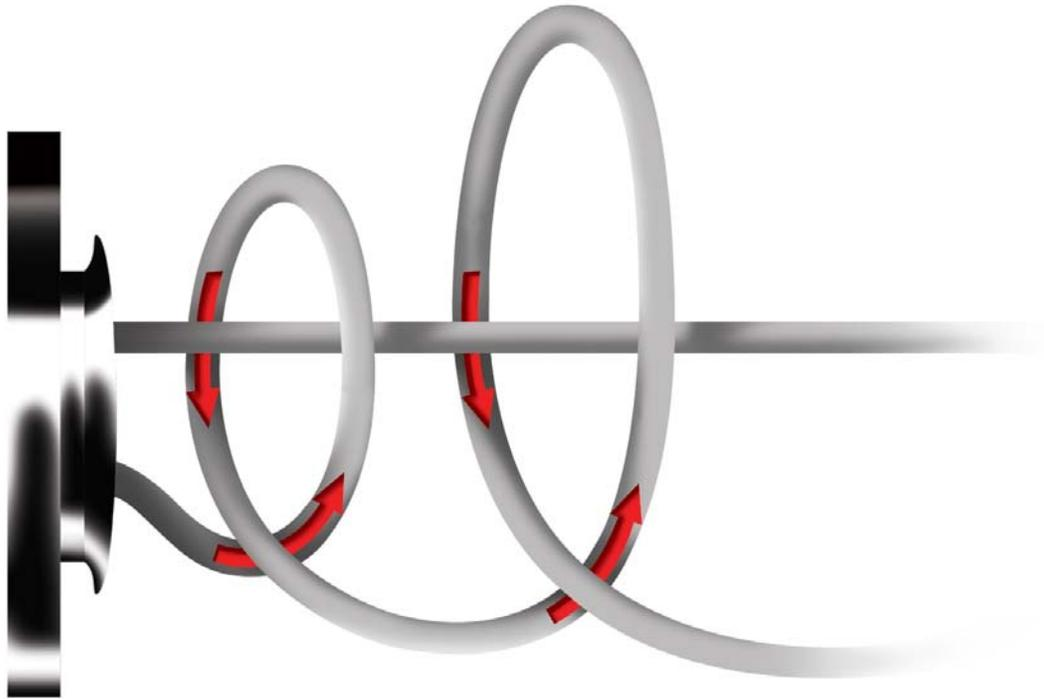
Use your needle-nose pliers to pull the knot tight. Pull side-to-side.
