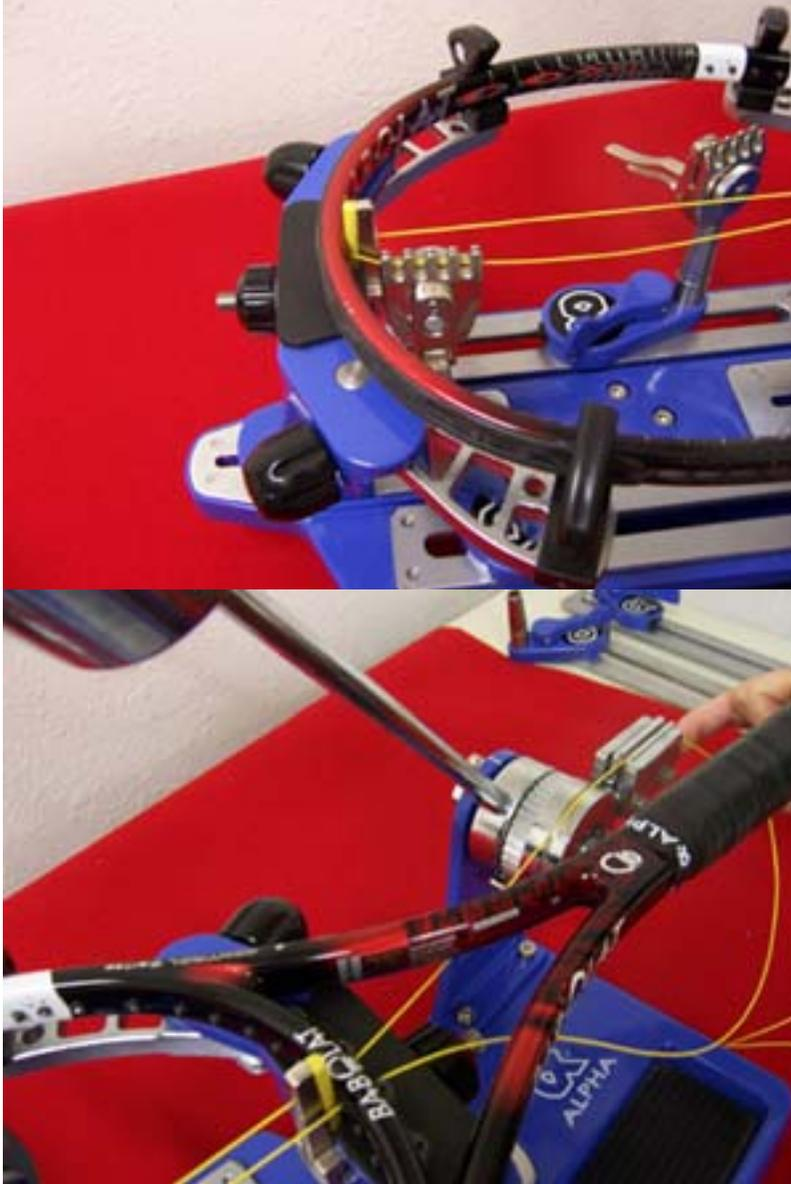
Step 4: Run the string under the beam of the racquet as picture above. *Before each pull rotate the gripper so that it is in the 1 o'clock position as shown below.*
